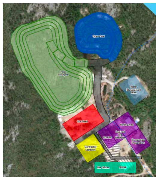
Figure 1: Approved site layout at North T Zone showing rock stockpile, ore feed, open cast pit and infrastructure
