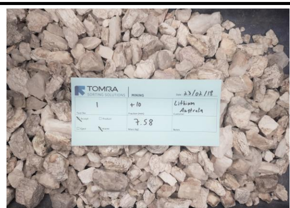
Figure 2: Ore sorting reject (mainly feldspar) from Lepidolite Hill mine dumps.
