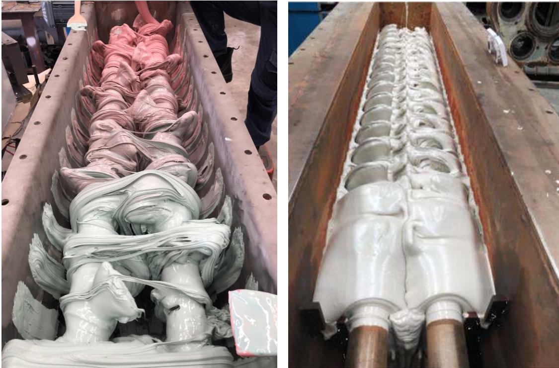
Figure 4 Sulphated Nolan's material being cooled in Gouda (L) and discharging (R)
