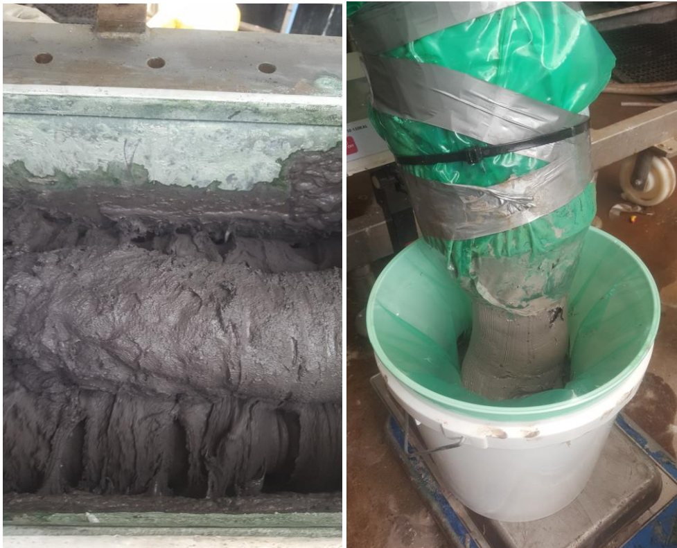
Figure 4 Sulphated Nolan's material being cooled in Gouda (L) and discharging (R)
