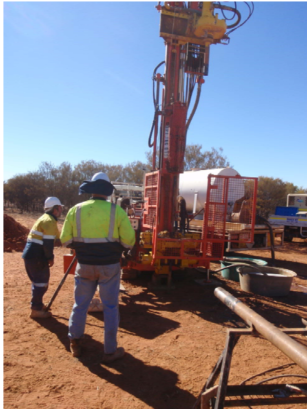
Geotechnical drillers completing Standard Penetration Test
