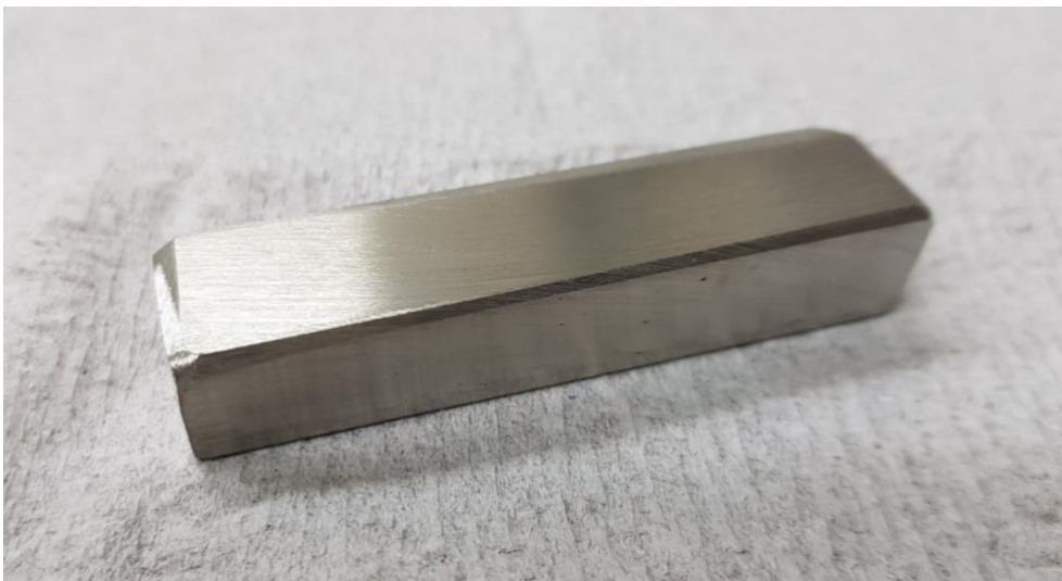
Figure 1: Neodymium : Praseodymium Metal Alloy - 9 kg @ 99.65 %
