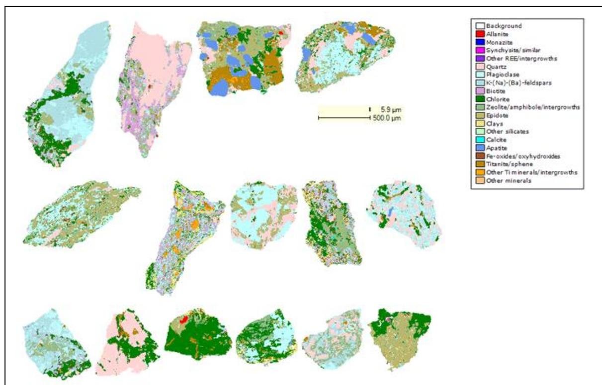
Figure 1: QEMSCAN Mapping of La Paz Mineral Assemblages
