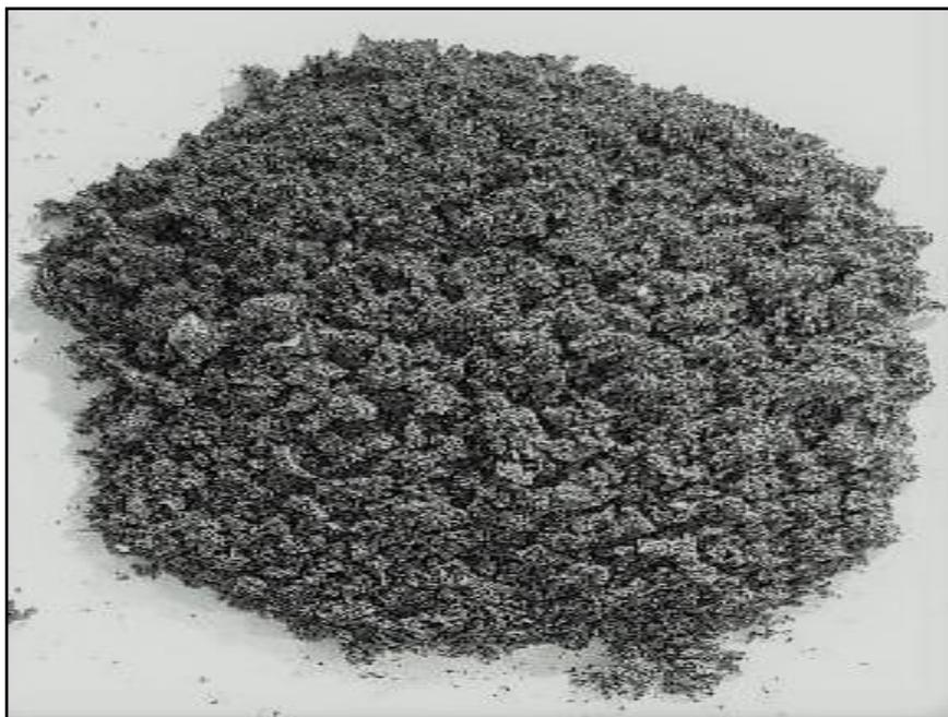
Figure 1: High Purity 99.8% Titanium Metal Powder
