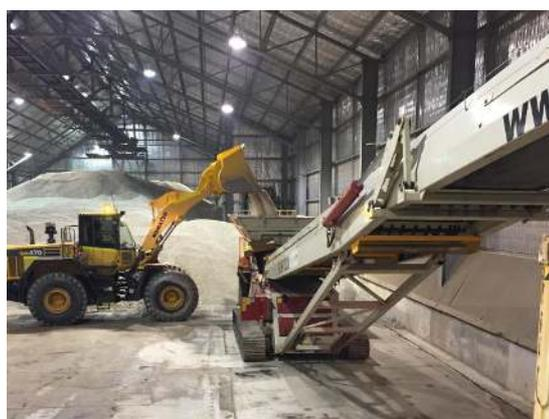
**Spodumene Concentrate being loaded at Port.**
