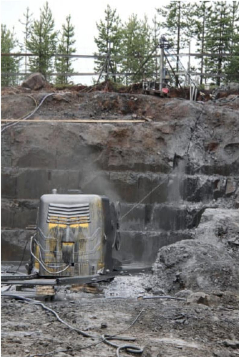
Slicing large blocks of graphite for dispatch reminds one more of stone quarrying than the traditional mining techniques of blasting and fracturing the material for processing into a concentrate. The advantage comes here from the grade of the
