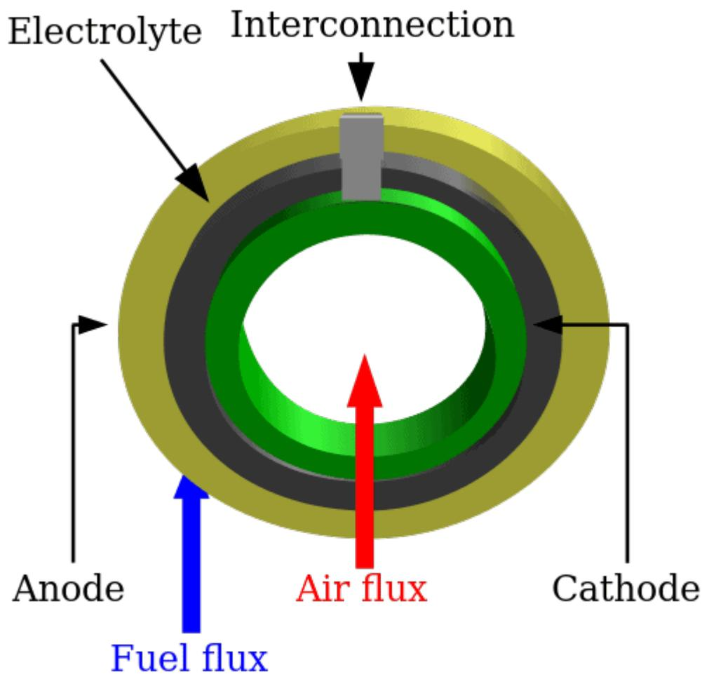
Incorporation of scandium in SOFCs enables a lower operating temperature resulting in longer lived equipment and less costly materials of construction. Bloom Energy in the US is the leading SOFC manufacturer and currently the single largest scandium user. The fuel cells are massed into stacks to match the energy required so the potential is enormous and once again limited only by the reliable supply of Scandium rather than any lack of potential end demand.
