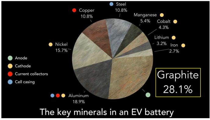
The key metals and minerals in a battery of an electric vehicle
