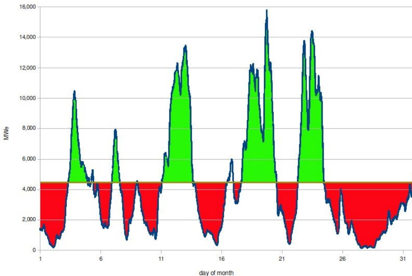
Figure 1: German wind generated power from January 2009. Red shows power output from storage systems that along with the power stored (green) would result in a constant power output.
