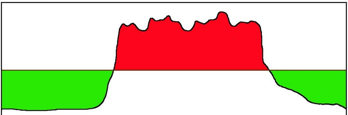
Figure 3: Typical commercial daily electrical consumption over a 24 hour period. Green shows local battery storing power and red indicates battery output of power in order to create an even consumption of power with time.
