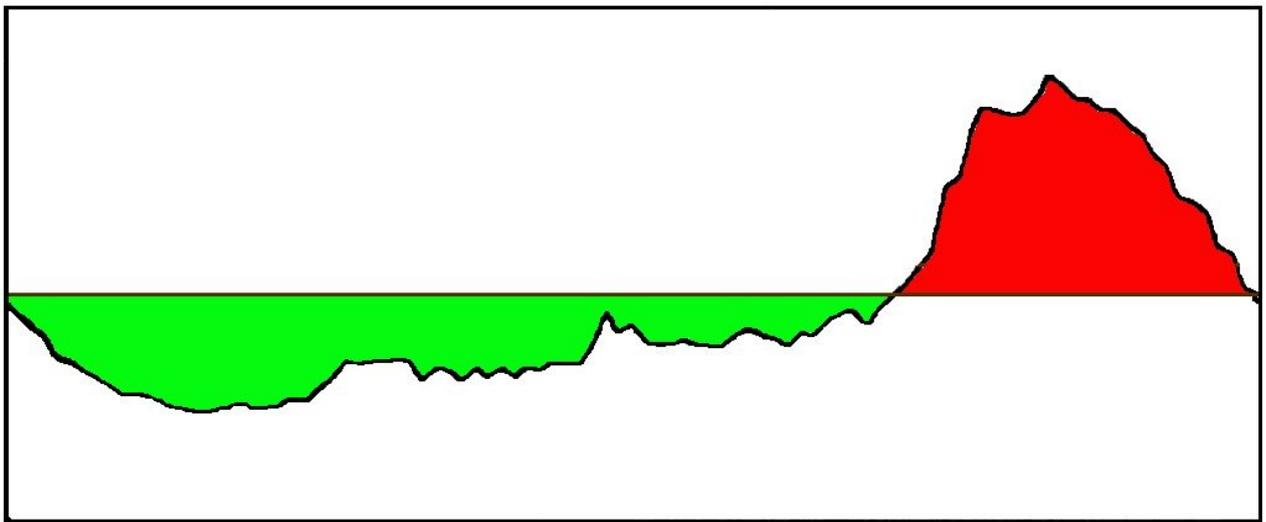
Figure 2: Typical residential daily electrical consumption over a 24 hour period. Green shows local battery storing power and red indicates battery output of power in order to create an even consumption of power with time.
