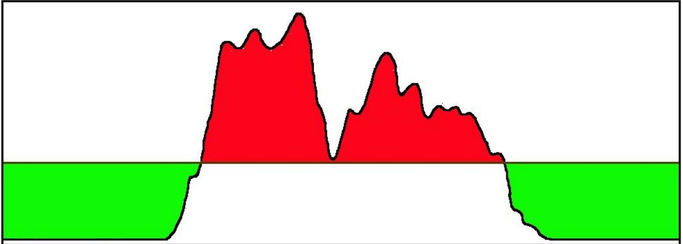
Figure 4: Typical small industrial daily electrical consumption over a 24 hour period. Green shows local battery storing power and red indicates battery output of power in order to create an even consumption of power with time.
