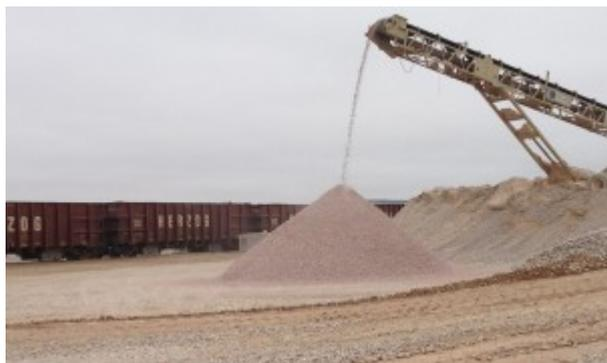
The photograph on the left shows the result of actual “Cryolite-Enriched and Rare Metal-Bearing Rhyolite” mined from Round Top Mountain in Hudspeth County in Southwestern Texas being “lightly” crushed at the base of Round Top, by equipment in place
