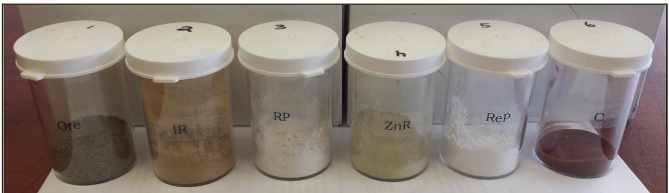
The process starts with finely crushed ore (vial 1 on the far left). The ore is then treated with acid, heated to 1800 C and then water leached. The pH is then raised to precipitate iron to give an orangey stained residue (as seen in vial 2). This is the major solid product from the process and it is 'dry stackable' to give a stable, compact residue impoundment.
