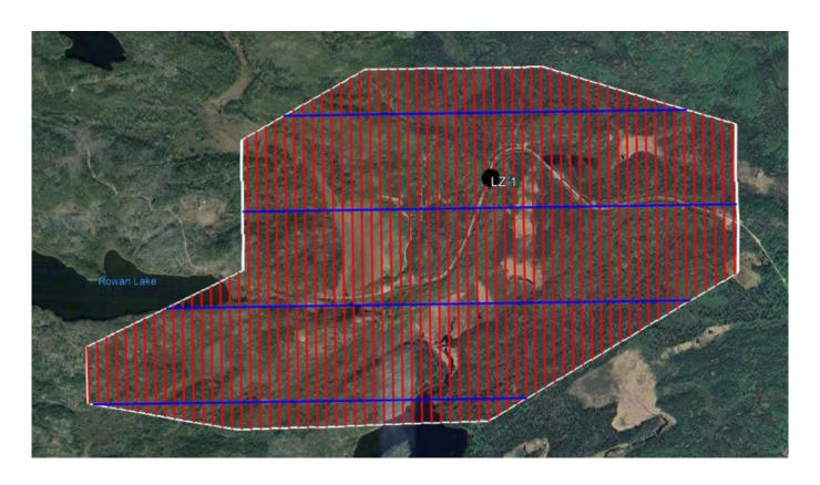
Survey Lines are Spaced 50 metres Apart
