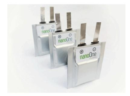
The LNM cathode  $(\text{LiNi}_{0.5}\text{Mn}_{1.5}\text{O}_4)$  was tested with a graphite anode and conventional electrolyte in a 20-layer pouch cell (4.75V 126mAh 0.592Wh) charging and discharging 12 times per day for 1000 cycles at 25°C and for 500 cycles at 45°C. This demonstrates enhanced durability under operating conditions that are relevant to automotive, power tool and energy storage applications in a cobalt-free, high voltage battery.
