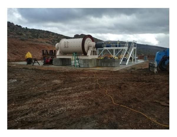
The ball mill as installed, on the mill pad poured by SBMI for this purpose.
