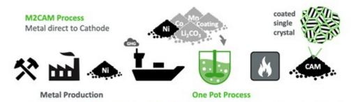
Nano One's Patented One-Pot Process and M2CAM enables cathode materials (CAM) to be made direct from metal by combining metal and lithium conversion, PCAM, CAM and coating into one reaction, eliminating the economic and environmental cost of metal sulfates and lithium hydroxide.
