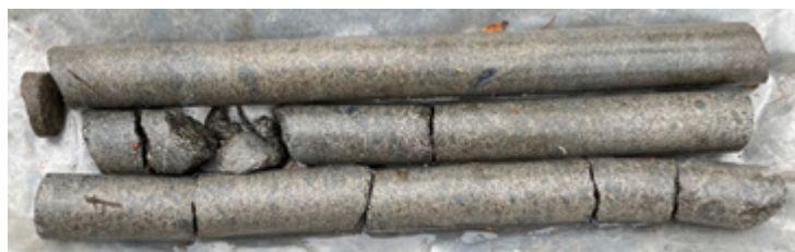
Figure 1 – 1.08 metre backpack drill core from PYC displaying semi-massive sulphide mineralization
