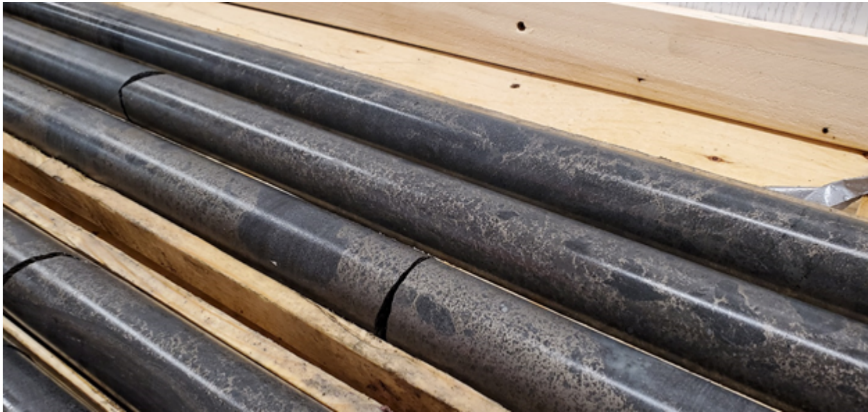
Figure 2: Semi-massive and breccia pyrrhotite mineralization observed in hole PYC21-001
