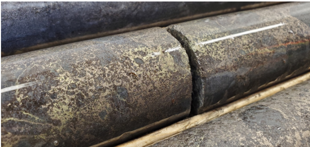
Figure 3: Close-up of pyrrhotite and chalcopyrite mineralization within hole PYC21-001.
