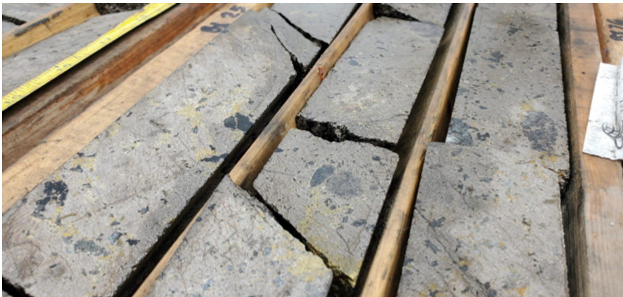
Figure 2: Drill core from BDF with observable pyrrhotite (iron sulphide), chalcopyrite (copper sulphide) and pentlandite (nickel sulphide) mineralization from an interval in Hole HPM08-04 which assayed 1.74% Ni, 0.66% Cu and 0.09% Co over 15.06 metres.
