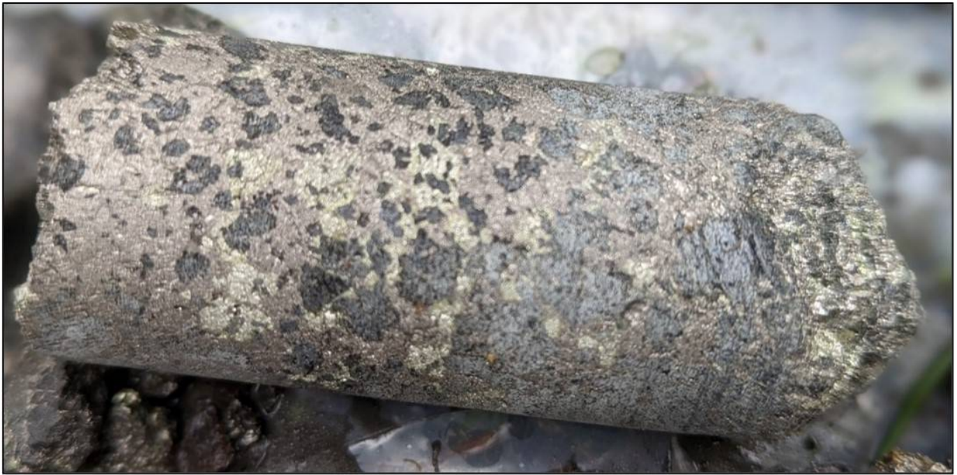
Figure 2: Closeup of mineralization in backpack core from the Taureau showing with semi-massive sulphide (pyrrhotite and chalcopyrite) mineralization.
