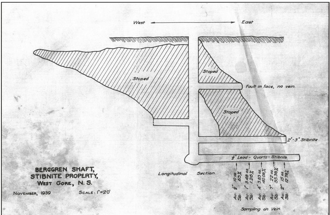
Figure 1: Cross-section of Berggren Shaft, showing historic sampling on vein
