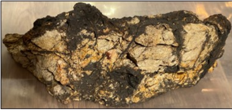
Photo 4: Sample Adit-01 Grading 189 g/t AgEq (41 g/t Ag, 4.83% Pb, 0.23% Zn, 6% Mn)
