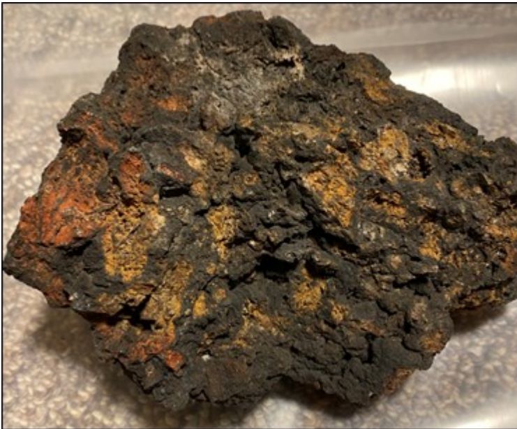
Photo 3: Sample Adit-05 Grading 253 g/t AgEq (180 g/t Ag, 1.5% Pb, 0.67% Zn, >10% Mn)
