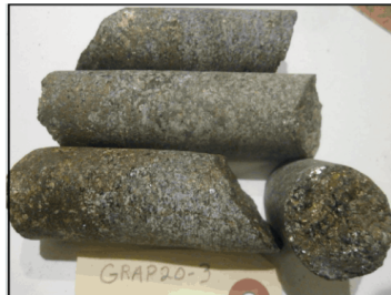
Figure 4. (3.2cm-diameter Core) Sulphide mineralization in Verification Core of Grand Portage showing (CNW Group/Canada Silver Cobalt Works Inc.)
