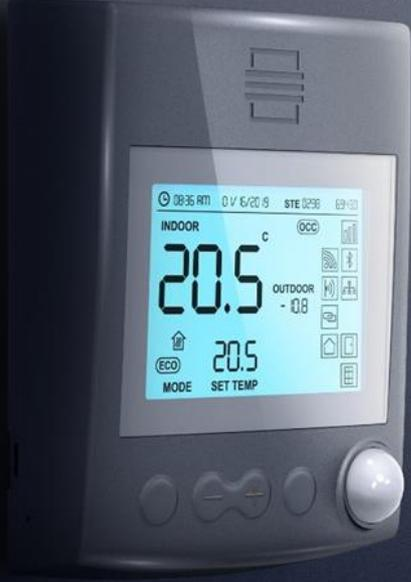
The image shows a SmartSuite thermostat with a color LCD screen. The screen displays the time 08:35 AM, date 01/15/2018, and STE 0230. It shows indoor temperature at 20.5°C, outdoor temperature at -0.8°C, and a set temperature of 20.5°C. The screen also features icons for various settings like OCC, ECO, and MODE. Below the screen are several physical buttons and a large circular knob.
