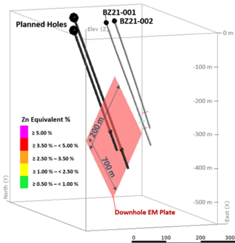
**Figure 1:** Oblique view looking north-northeast of the 2021 Betty Zone drill holes displaying Zinc Equivalent percentages as derived from assays, the interpreted electromagnetic plate from the downhole geophysical survey, and the planned holes for the summer 2021 drill program.
