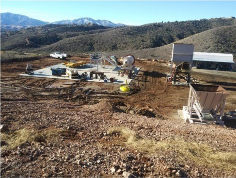
*Overview of SBMI's mill site, showing the fine and coarse ore bins on the right, the ball mill in the middle, and assorted equipment to the left.*
