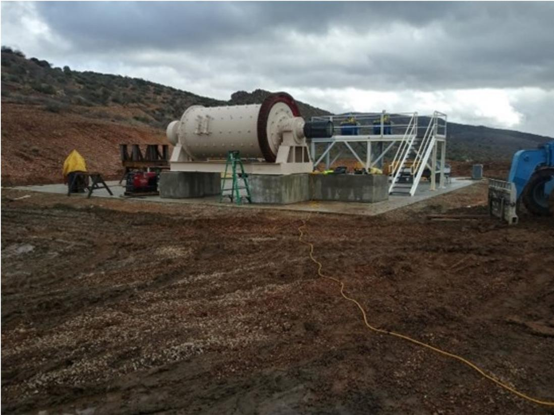
*The ball mill as installed, on the mill pad poured by SBMI for this purpose.*
