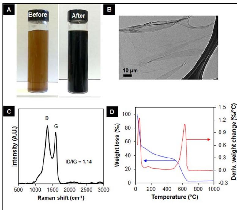
**Figure 1.** A) Images of graphene oxide (GO) before and after the reduction process, B) TEM image of a reduced graphene oxide (rGO) sheet, C) Raman, and D) TGA plots of rGO reduced from GO using amino acid.
